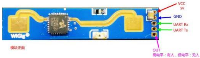
Figure 6 Module pin definition diagram
